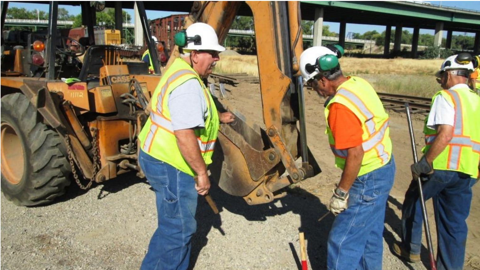
Harry and Ed take on some quick-fixes to the keeper-ring on the pivot pin of the back-hoe
