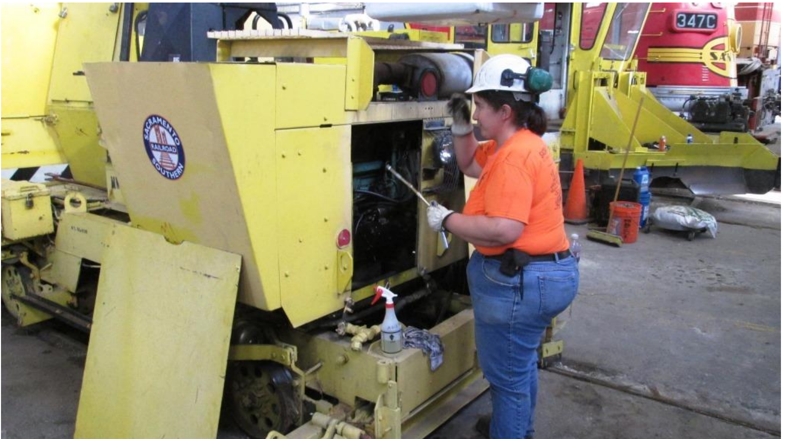
Heather replaces the man-lift's starter
