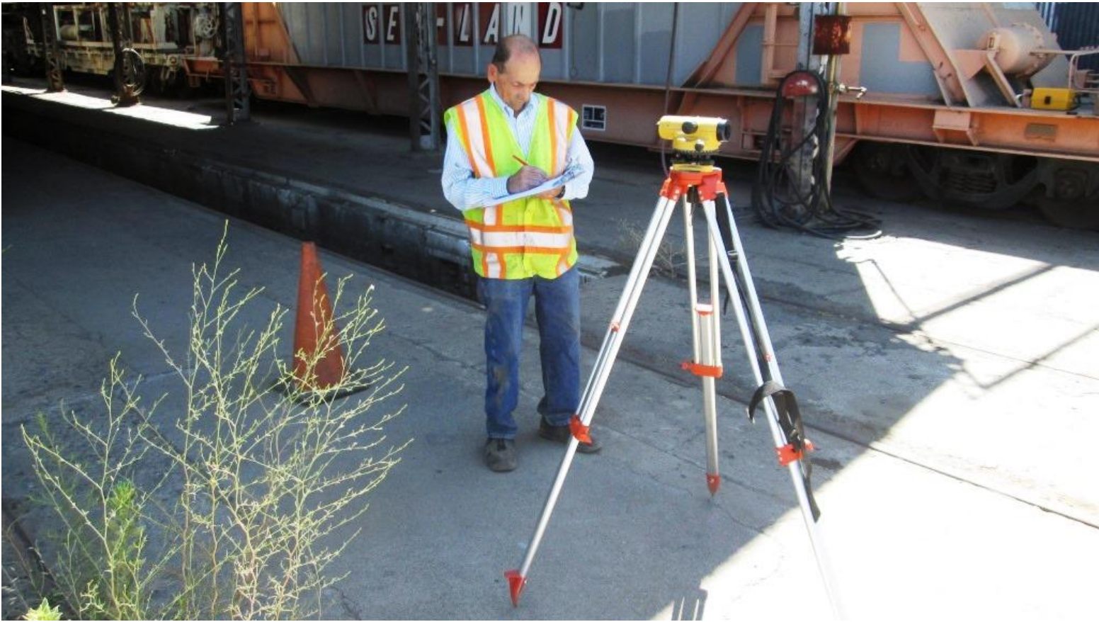
Harry G. sights the placement of the track
